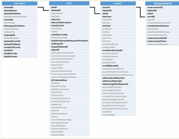
Figure 2. Graphical representation of the structure of the SPARSE database, with the four central tables (indicated by numbers). Fields for which data must be entered (i.e. required fields) are marked by bold black letters. Fields that are optional are marked by regular grey letters.
